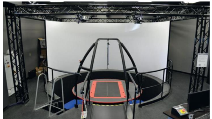
Figure 1: CAREN system is comprised of a split-belt treadmill on a tilting base, real time motion capture, and a 120-degree surrounding projection screen.
