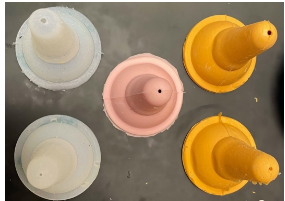
Figure 1: Custom fabricated nipples were used in this study. Compliant nipples (left, white) and stiff nipples (right, orange) were tested along with large hole size (top) and small hole size (bottom). A training nipple (middle, pink) of intermediate stiffness and hole size was used for all other feeds.
