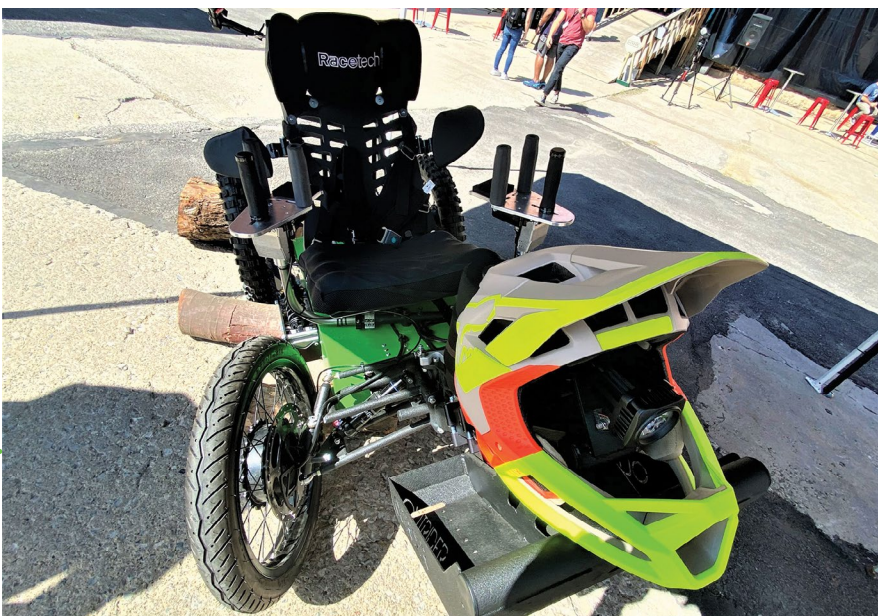
Mountain bike outfitted with electric power steering unit. The bike was the Adaptive All-Terrain Motorized Trail Vehicle' Senior Design project led by Steve Wilson and student team. See Page 30.
