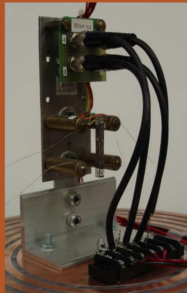
Figure 1: Experimental setup photo of vibrational beam gyroscope and rate table
