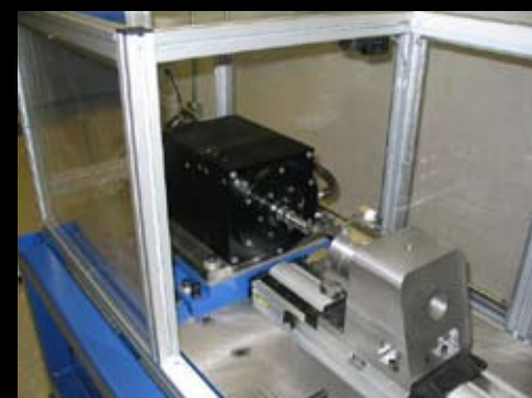
Figure 1: AMB-supported high speed machining spindle.
