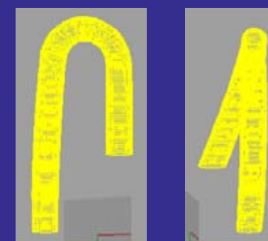
Figure 4: Image-based reconstructed geometry of an aortic model, showing the aortic arch (left) and the non-planar nature of the geometry (right).
