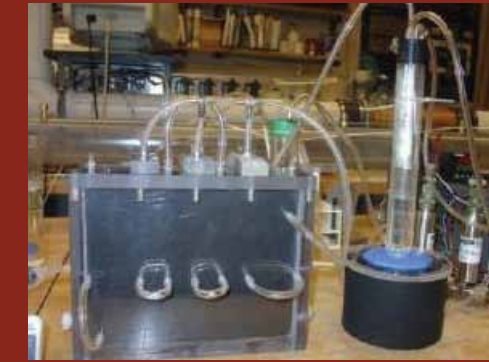
The 3-T apparatus for selective phase separation experiments.
