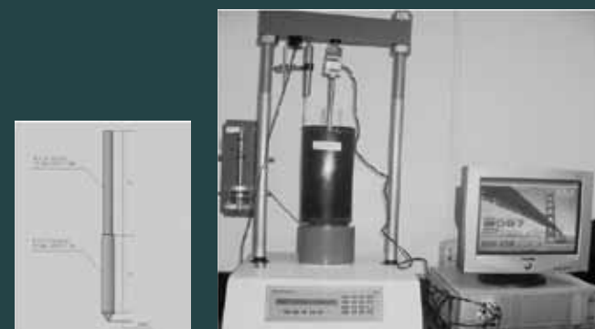
Static Load Test of Piles
