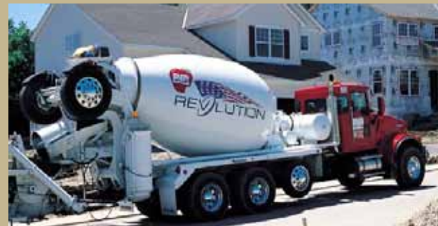
REVOLUTION COMPOSITE DRUM: This innovative concrete mixing drum gives ready mix producers the competitive advantage by being able to carry more concrete per load. It is also two thousand pounds lighter and has twice the durability of similar steel drums. The end result being that fuel is conserved and jobs are getting done faster.
