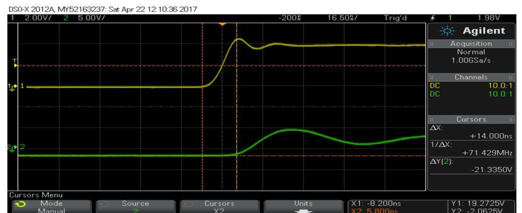
Figure 3: Simulation & Propagation Delay for Front End Circuit
