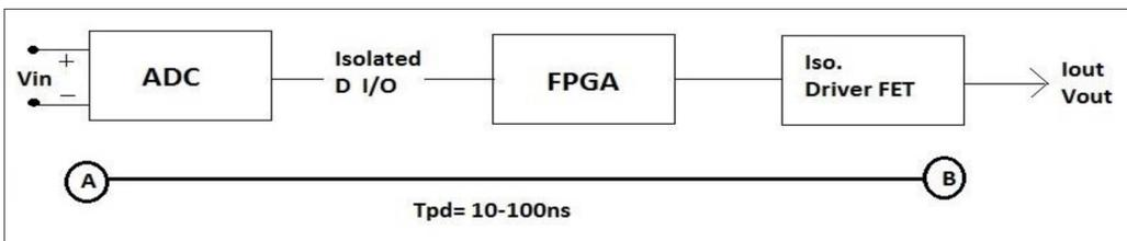
Figure 1: Signal Conditioning Circuit Feedback Loop
