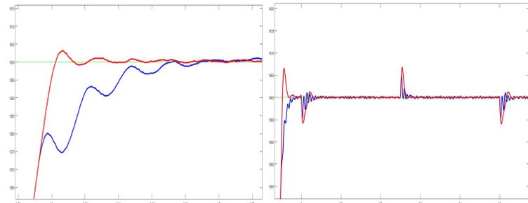
Figure [5]: ADRC vs tuned PI (Sinusoidal Disturbance)
