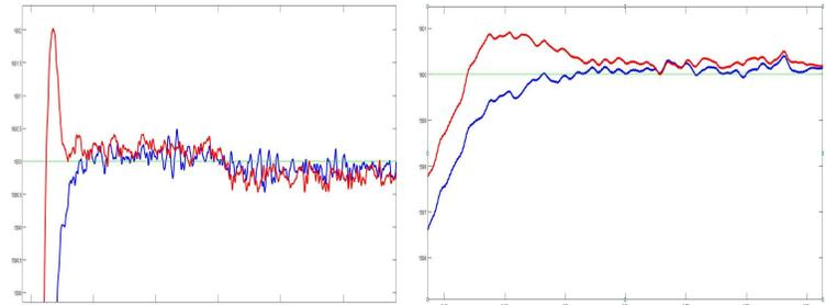
Figure [4]: ADRC vs tuned PI with an increased internal resistance (x2 left, x3 right)
