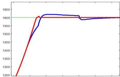
Figure [3]: Untuned PI controller vs. BBO tuned PI controller
