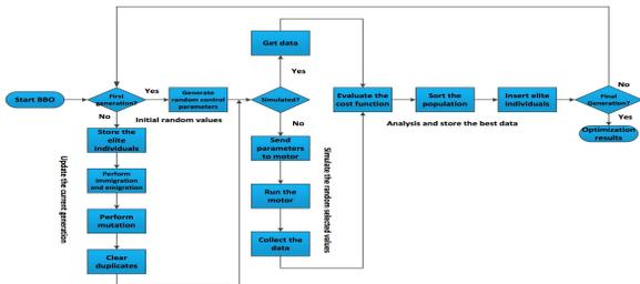
Figure [1]: BBO For DFIMotor Control Mechanism
