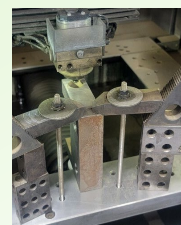
EDM Holes for Press Fit Bushings
