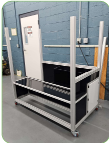
Aluminum extrusion with aluminum plates and clear/black acrylic sheets for enclosure
