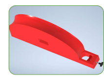
Mandrel with clamping mechanism holds and bends hose to required radius
