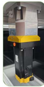
Motor & Gear Box provides power, modifies motor's speed and torque
