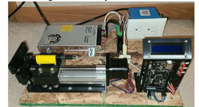
Fig 8: Linear Rail Testing Apparatus
