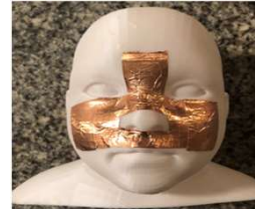
Fig 7: 3D Model with Conductive Layer
