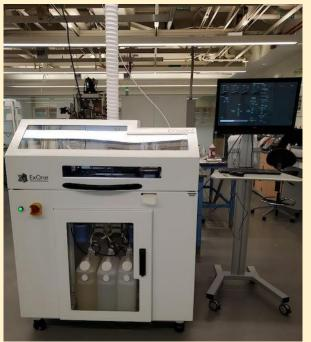
This is an industrial-scale printer with an ability to print a variety of powdered materials, including stainless steel, iron, bronze, tungsten, glass and can be configured to print other materials. The printer has the following specifications:
